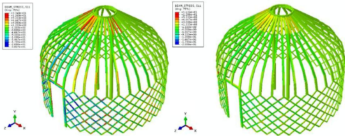
Figure 7. Longitudinal stresses on the Lodge beams - wind speed of 140 km/h, measured on site on the 24<sup>th</sup> February. Left: without rock wall; right: with rock wall.
